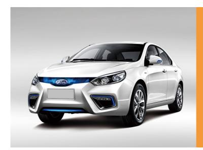
Through nine months, JAC new energy vehicle R&D team developed one platform with three models A-class pure-electric vehicle. It has a long life and high-ration ternary liquid-cooling battery system and the maxima driving range reaches 500km. In the process of R&D, manufacturing, marketing, planning, technology and design have a very effective combination to complete iEVA50 's developing and producing. The taxi of this model have been put into operation in Hefei.
